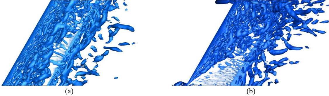
Figure 4. Instantaneous iso-surface of the second invariant of the velocity gradient tensor ( Q = 5000 ): (a) periodic boundary conditions and (b) wall boundary conditions ( \beta = 30^\circ , U_r = 11.5 ).
